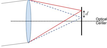
**Fig. 1.** Lateral chromatic aberration (LCA). The symbol  $d$  denotes LCA displacement.
