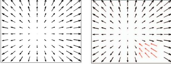
**Fig. 2. Left:** Lateral chromatic aberration (LCA) displacement vector field for an authentic image. **Right:** LCA displacement vector field for a copy-paste forgery, with pasted LCA in red. Displacement vectors are scaled 200X.
