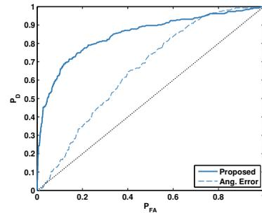
**Fig. 5.** The receiver operating characteristic for detection of copy-move forgeries created radially using images from the CER camera.
